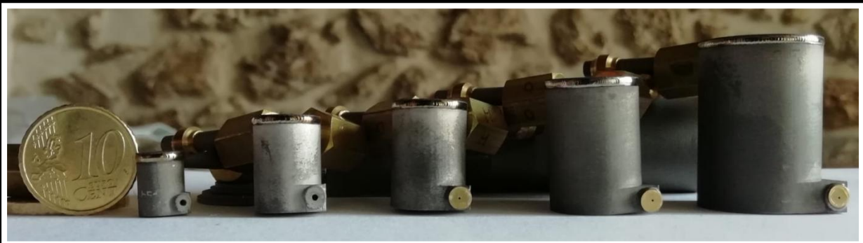
Figure 1 - Thrust chambers (from 6x9mm, left, to 20x30mm, right)
